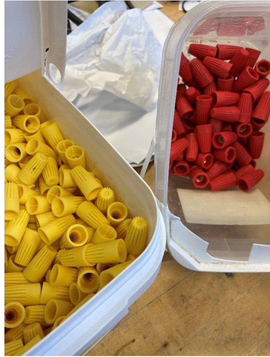
Twist-on wire connectors, also called marettes.
